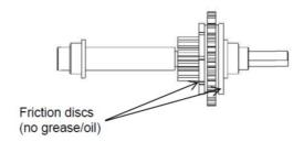
2. Apply a drop or two of #30 weight engine oil to each bushing I.D. and to the ratchet pawl pivot points. Maintain a thin layer of chassis grease on the gear teeth.
